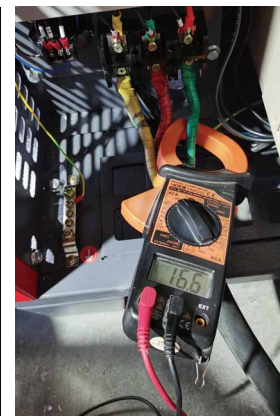
Voltage and current detection
